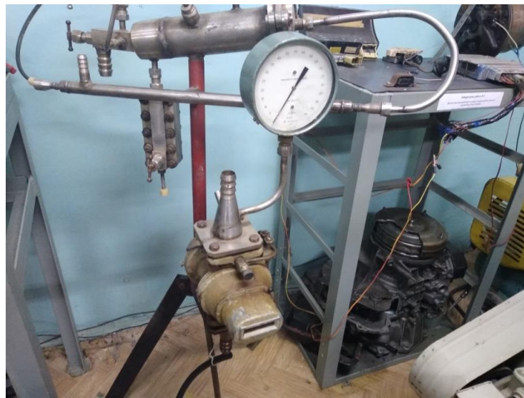
Figure 4 – A flow meter for measuring the volume flow of exhaust gases and a manometer for determining the gas pressure
