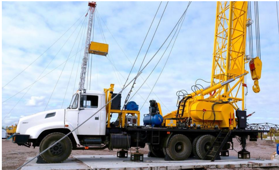
Figure 10 – AORS-60 model well-repair lifting unit
