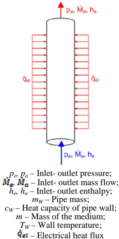
Figure 3 – Model for describing a boiling process
